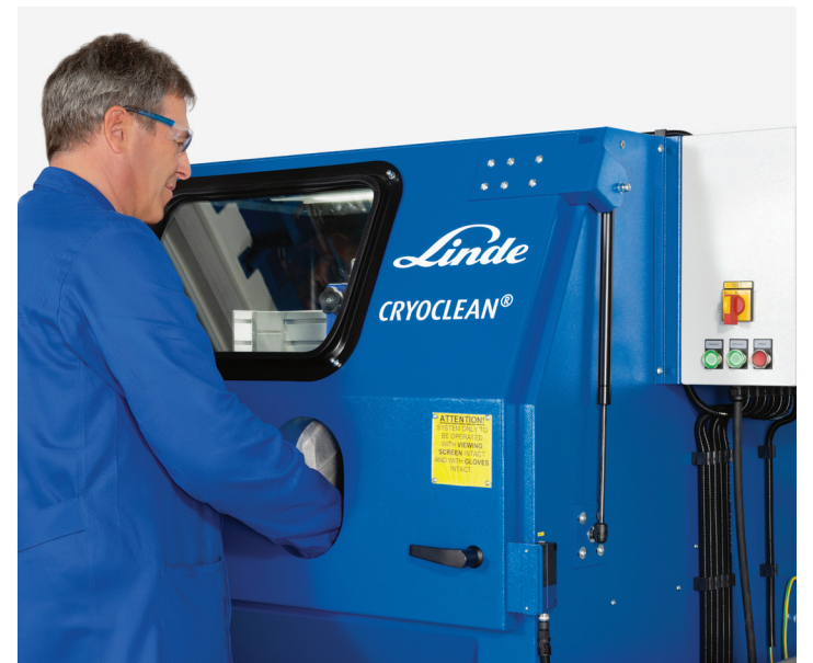
ADDvance Cryoclean uses dry ice particles (CO 2 snow) to clean the products after printing
